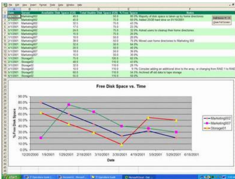
Figure 2. You can track disk usage over time using a simple Excel spreadsheet and Windows 2000's Computer Management tool. (Click image to view larger version.)
